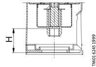
Fig. 1 Clearance of the pump shaft
