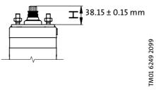
Fig. 2 Shaft height of the motor
